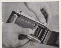
out a few inches of the film and insert the film leader into the slot of the take-up spool 5 making sure that the sprockets 4 properly catch the perfora-
